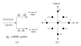
**Fig. 2** (a) The STBC encoder block diagram and (b) is a 9-point signal constellation, that is air combined two transmitted QPSK symbols from Ant. #1 and Ant. #2 in one QPSK symbol period.
