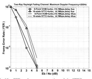
**Fig. 10** FER performance comparison of the STTC concatenated turbo code OFDM scheme and the 8-point VCM OFDM scheme in the two-ray fading channels.
