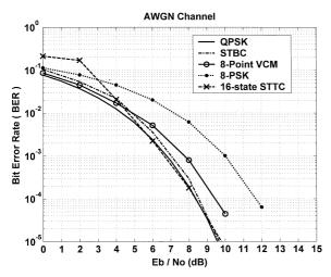
**Fig. 4** The BER performances of the 5 different transmit schemes in AWGN channel. The 8-QASK BER performance is the same as the 8-point VCM case.
