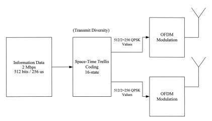
Fig. 7 The OFDM downlink 2 Mbps framework employs a 16-state space-time trellis code [8].
