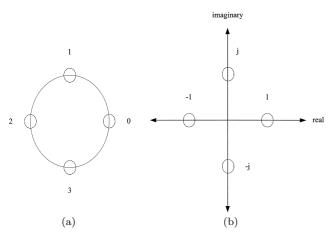
${\bf Fig. 1}$   $\ \ (a)$  The QPSK signal constellation and (b) is its real and imaginary part.
