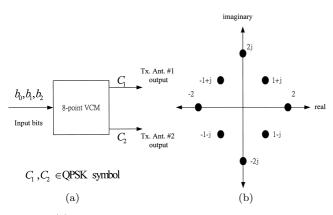
Fig. 3 (a) The virtual constellation mapping function block and (b) is the 8-point signal constellation.
