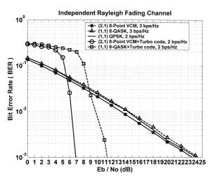
**Fig. 5** The BER performances of the 5 different transmit schemes in Rayleigh fading channel. The turbo coded frame length is 512 bits, and decoding iteration number is 4.
