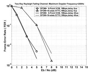
Fig. 9 FER performance comparison of the 8-point VCM OFDM scheme and the STTC OFDM scheme in the two-ray fading channels.
