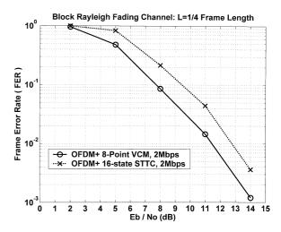
Fig. 8 FER performance comparison of the 8-point VCM OFDM scheme and the space-time coded OFDM scheme in the block Rayleigh fading channel.
